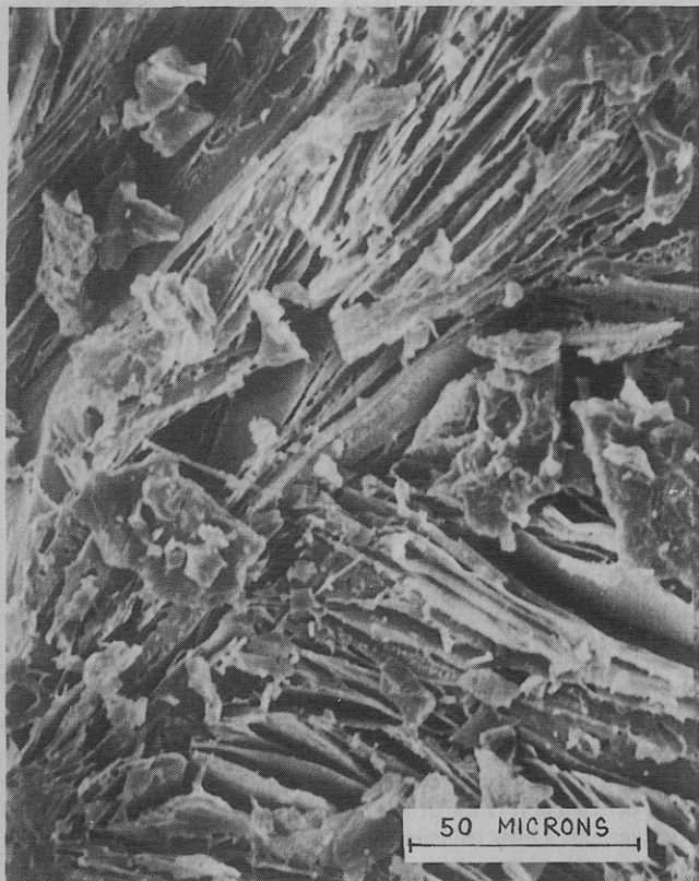
Figure 1. Scanning electron microscopic picture of a freeze-dried 50/50 PS/PMMA particle surface. The original print magnification was 630 \times .
